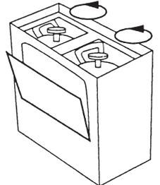
By turning the valves **COUNTER CLOCKWISE** open both valves completely. Top flap may be removed or left in place during use or storage.
