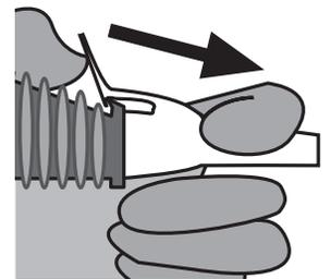
To remove used nozzle, push top latch up and forward to unsnap.
