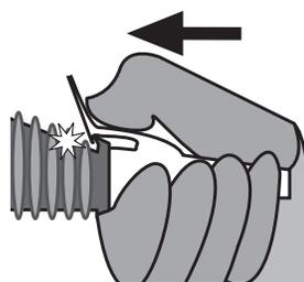
Attach top latch by pushing towards back of unit, until an audible "snap" is heard.
