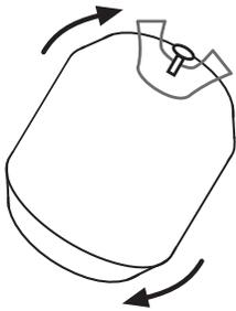
Invert each cylinder several times before use to insure proper mixing.
