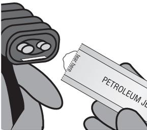
Before attaching nozzle, use petroleum jelly on face of gun. After attaching nozzle, spray into "test shot" receptacle. Unit is ready to use.
