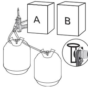
Thread red coded hose to A-component tank and black coded hose to B-component tank and tighten with a 9/16" wrench.
