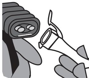
Insert bottom tab of nozzle into bottom slot of dispensing unit.
