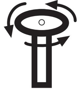
By turning the valves **COUNTER CLOCKWISE** open tank valves completely. Tank valves must be upright during use.
