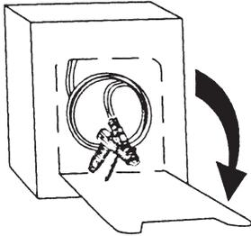
Push in top of front panel to open. Pull down flap for dispensing unit hose assembly. Remove nozzle packet and read instructions.
